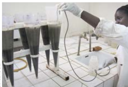
Photo 1: Settling experiments with faecal sludge in Dakar, Senegal.
