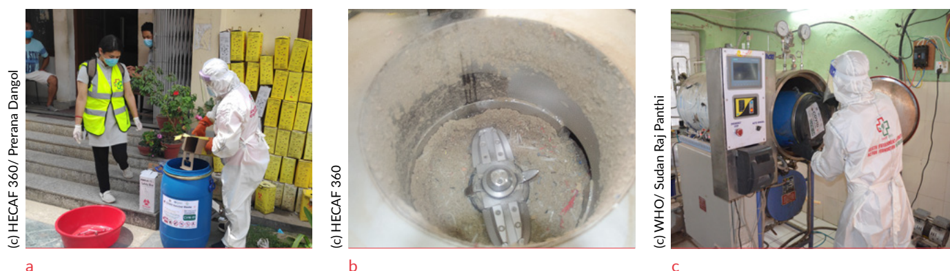
FIG. A6 — (a) Collection of safety boxes in drums. b) Shredded waste after microwaving. c) Loading of the autoclave.
