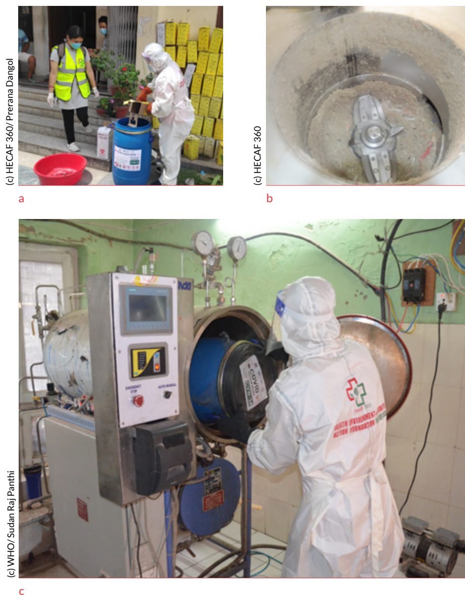
FIG. A6 – (a) Collection of safety boxes in drums. b) Shredded waste after microwaving. c) Loading of the autoclave.
